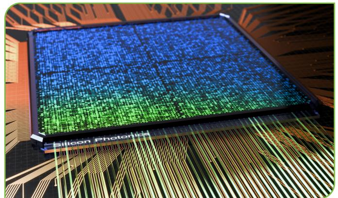
combines numerous individual electronic components onto a single substrate, PICs integrate multiple photonic components onto a single substrate. The use of photonic, rather than electronic, components offer significant advantages in speed, energy efficiency, and data capacity over traditional microelectronic components.
